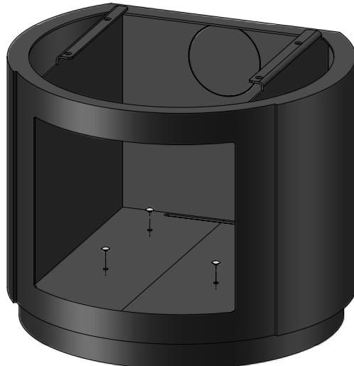
The assembled rail system is then fitted in their place as shown on the sketch using the 4 no. M6X10 hexagonal screws supplied.
